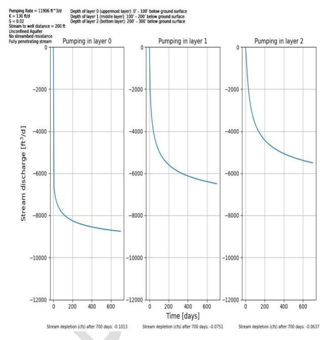
Figure 4-Simulation of Well Seal Depth Impacts on Groundwater Extraction at Different Depths (TTim, Bakker 2013)
