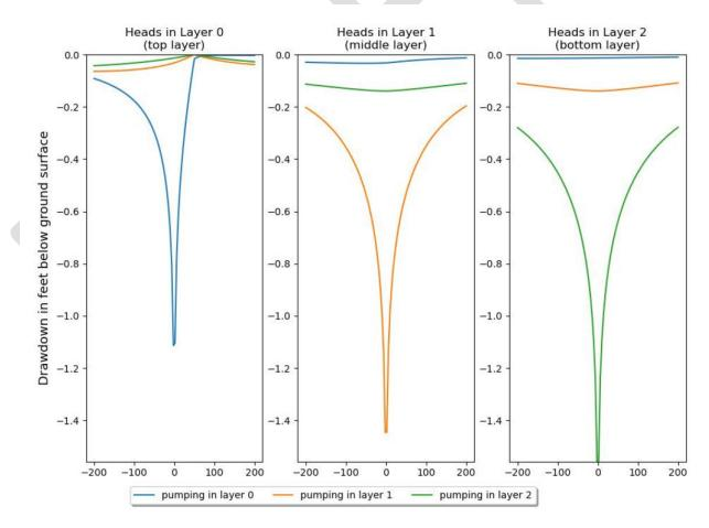
Figure 1- Drawdowns at Different Seal Depths (TTim, Bakker 2013)
